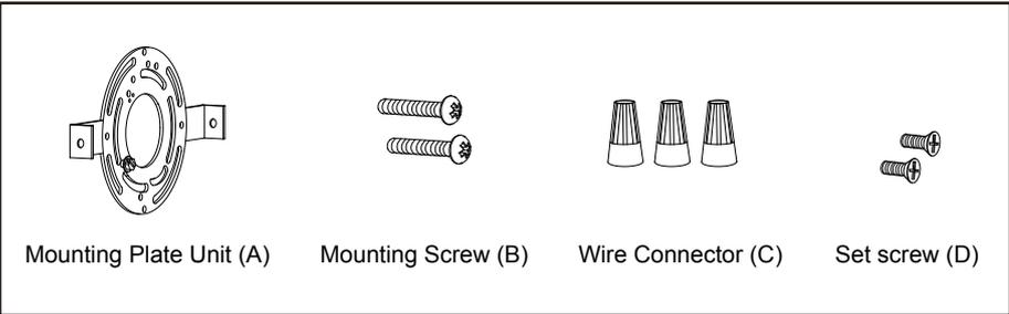
Mounting Plate Unit (A)    Mounting Screw (B)    Wire Connector (C)    Set screw (D)
